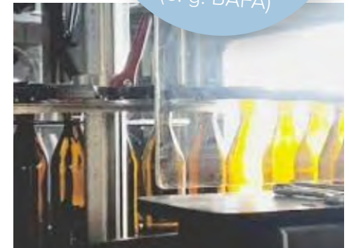
Blasting/Drying of bottles in front of optical inspection.
