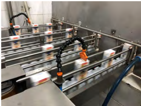
Blasting/Drying of drink packs in front of printing station.
